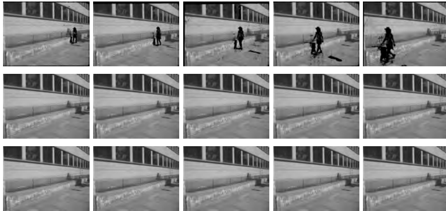
Fig. 3. At the upper row, foreground is in black. At the lower rows pixels were replaced with background estimation first and with the nearest neighbor second.
